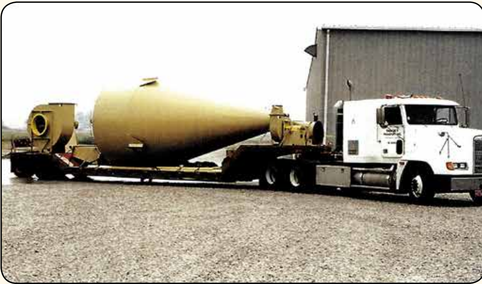
All welded oversized cyclone being delivered with main fan and relay fan.
