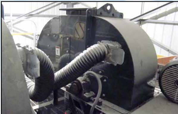
Dust collection suction ports on two bucket elevator head covers.
